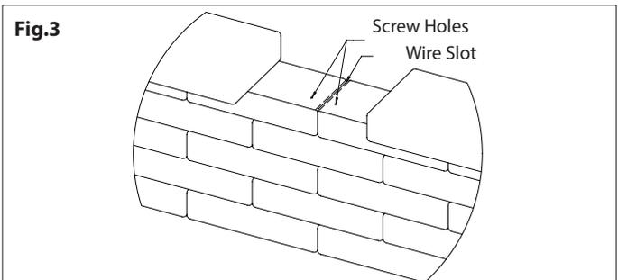
5. Checking the required drill size for your flush mount plastic anchors for No. 4 screws, use a hammer drill with a masonry bit to drill out two holes at the screw locations. The depth of the hole should be slightly longer than the length of the plastic anchor.
