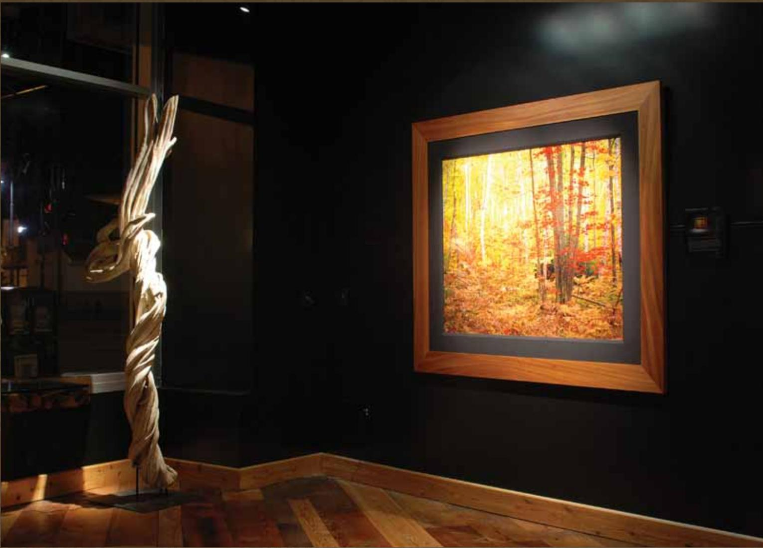
WAC MR16 track luminaires were used with Ushio MR-16 Eurostar™ IR Series of halogen lamps to provide the lighting intensity needed and to comply with California's Title 24 energy efficiency code.
